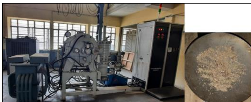
Fig. 2 and 3: Vacuum furnace and Thermal processed nanoparticles
